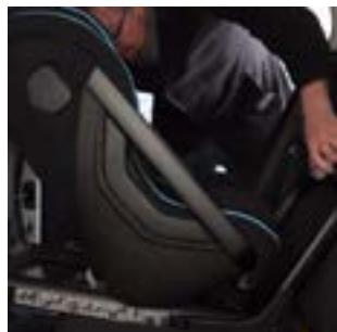
Quick & safe installation in 30 seconds – Simply click the seat into the vehicle's ISOFIX-Connectors, unfold the stand base and fix the automatic rebound bar. Done!
